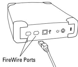
**Figure 5.** Connecting to a FireWire port
