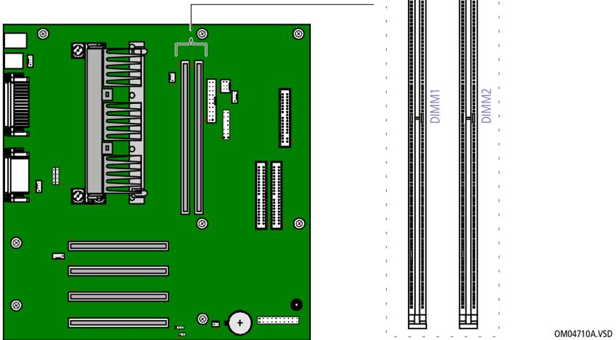
Both sides of each Dual Inline Memory Module (DIMM) look very similar. The side with pin 1 has a small "1" to the left of pin 1. Be sure to orient a DIMM correctly in the DIMM connector (a small triangle on the connector indicates pin 1).
